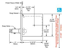
Rough Wall Opening 8-3/8" (210mm) wide 4-3/8" (110mm) high 3-7/8" (98mm) minimum recessed depth
